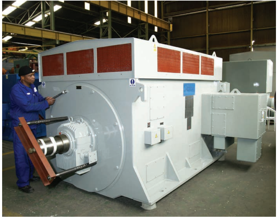
A IP22 IC01 3MW UNIBOX featuring a top mounted inlet cooling housing and a bottom exit design for the hot air. This design reached a performance efficiency of over 97%.
