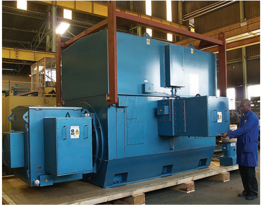
A large frame 7MW 11kV UNIBOX Slipring Mill motor being crated and prepared for export.
