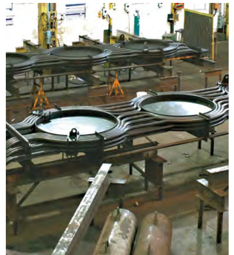
Boiler tube manipulation
