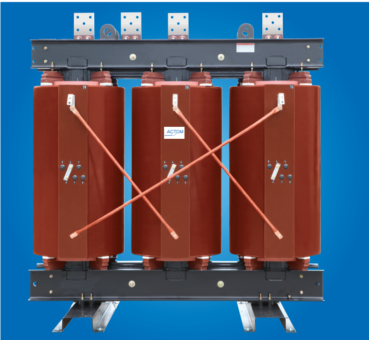
500kVA 11/0.4kV Dyn11 Cast Resin Dry Type Transformer.
