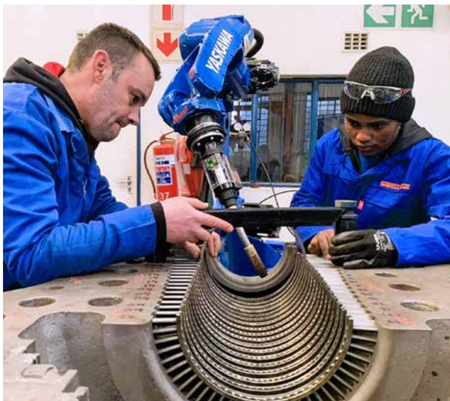
Steven Rudd (left), Metalplus' Workshop Supervisor, and Nsindiso Mzimela, Engineer in Training, are shown setting up the shroud bands for robotic welding on the top casing of the turbine.
