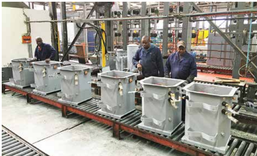
Distribution Transformers factory workers are seen above tanking 64kVA 22kV low-loss transformers as part of the new interim distribution transformers contract for Eskom.
