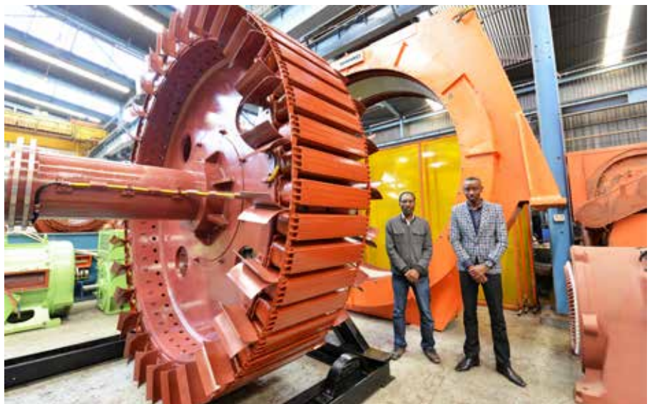
This 30 year old large 2150 kW synchronous mill motor was repaired by Marthinusen & Coutts for a Zimbabwean gold mine in 2017.
