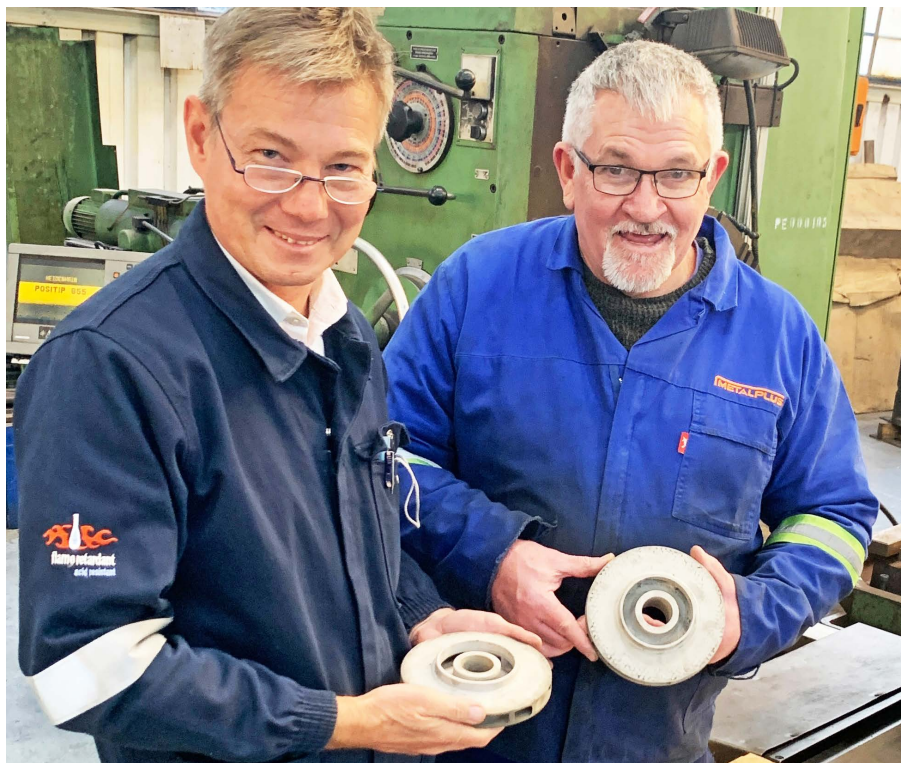
Metalplus' Divisional CEO Roman Mornau (left) and Senior fitter Charlie Pohl inspect two of the 3D metal printed impellers prior to machining.
