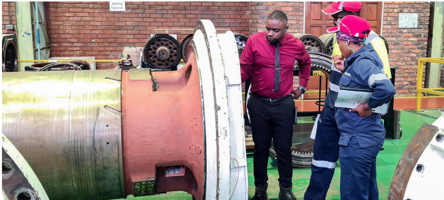
Reid & Mitchell Mechanical Engineer Sphiwe Sithole explains the workings of a 788 model wheel-motor for a Komatsu 730E dump truck to two Komatsu electro-mechanical millwright apprentices.
