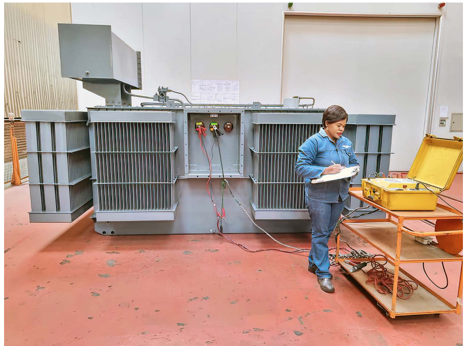
Khuliso Mutheiwana, Distribution Transformers' Chief-of-Test, is shown above conducting routine tests on a 5MVA power transformer in the division's Highbay test facility.
