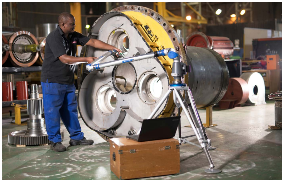
Thomas Siphiri, R&M's Mechanical Assessor, is shown above using a Faro arm for precision measuring to assess a refurbished 788 model wheel-motor for a large off-road dump truck.
