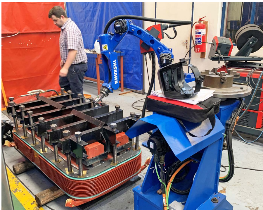
Metalplus' Quality Controller Ric da Costa keeps a watchful eye on the CMT robotic welder as it carries out complex weld procedures in repairing a salient pole core and retaining plates.
