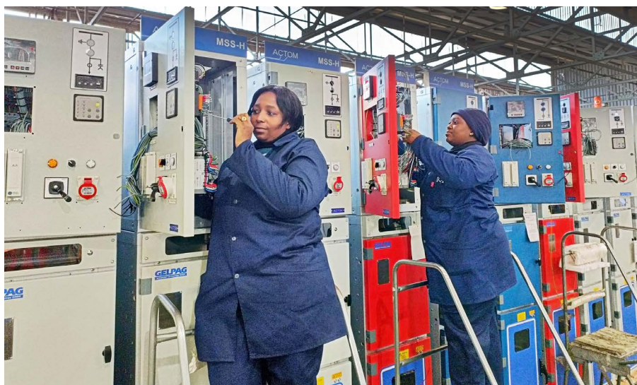
MV Switchgear wiring technicians Phyllis Morena (left) and Petra Maliga complete wiring of locally manufactured LV compartments fitted onto GELPAG SIS switchgear panels due for installation in underground substations at Kamoakakula copper mine in the DRC.
