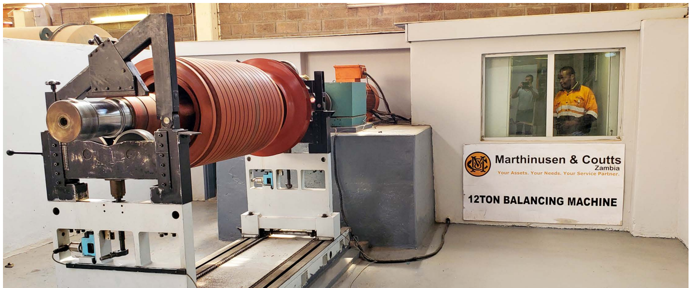
Senior Balancer Darlington Musonda is shown above balancing the rotor of one of the two compressor motors on M&C Zambia's 12t balancing machine.
