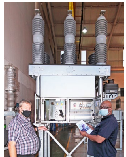
Craig Aaron and HVE's MV Circuit Breaker Foreman Alex Mudau with one of the new 36kV outdoor combo vacuum circuit breakers, branded CTB36Plus, that are now in production at High Voltage Equipment's Knights factory.
