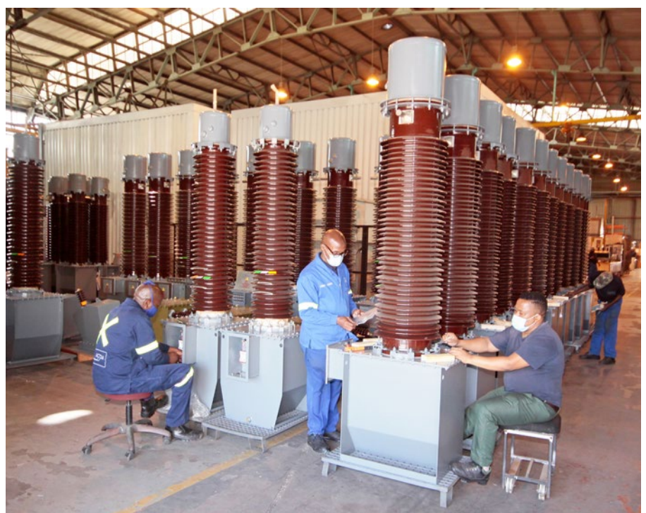
High Voltage Equipment assembly staff doing final checks on high voltage transformers to be installed in solar and wind farm sub stations.
