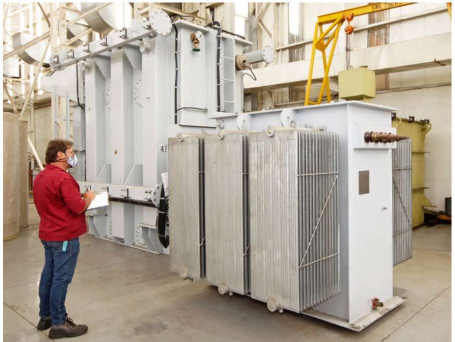
A 2.8MVA 0.69/33kV step-up pad mount transformer next to the much more significant 33/132kV step-up collector transformer for wind and solar applications - both supplied by ACTOM Power Transformers.
