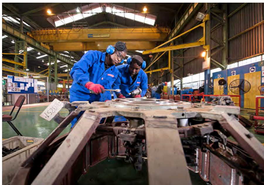
R&M Generator department prepares a locomotive main generator field frame before re-assembly.
