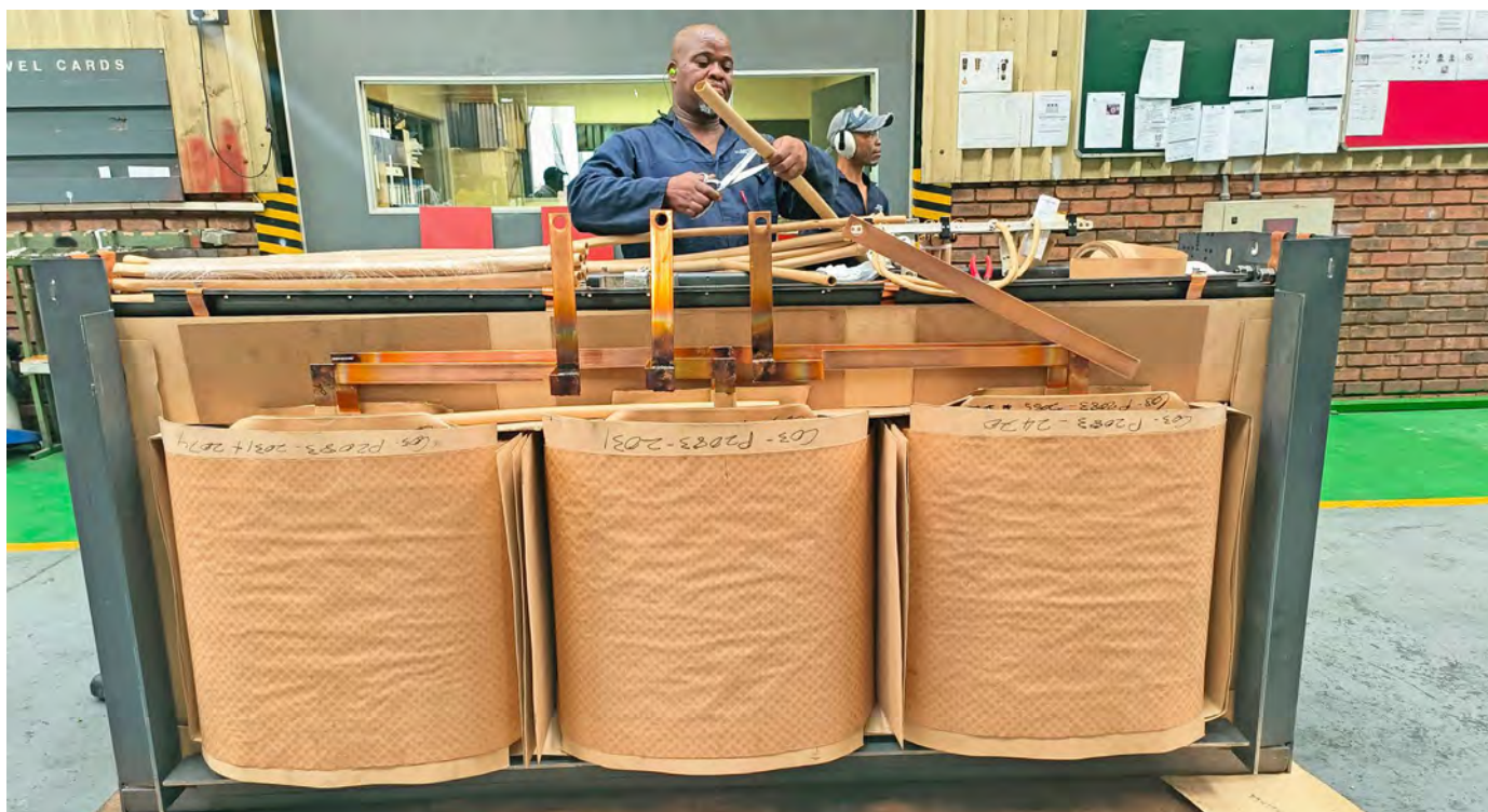
Sibusiso Ngobese, ADT Wireman preparing the active part of the transformer.
