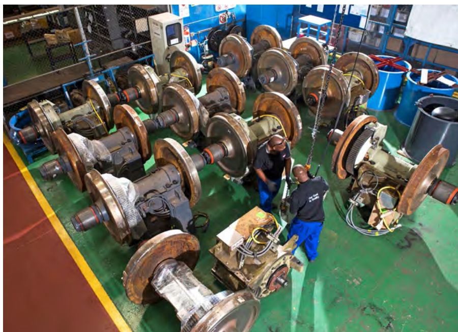
R&M Traction Department install AC Traction motors to locomotive wheelsets.
