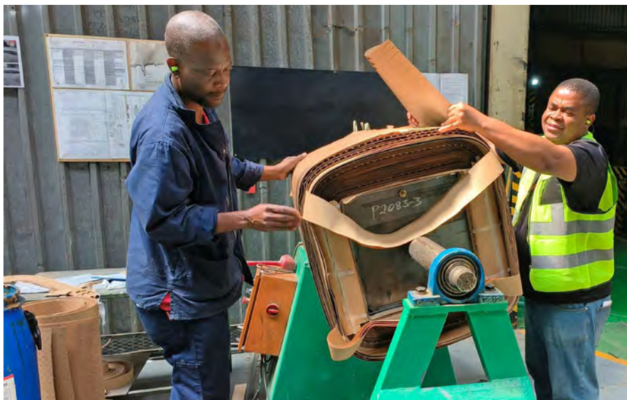
From left: Daniel Godi, ADT Winder and Geoff Nedzamba, ADT Chief Quality Inspector winding a transformer coil.
