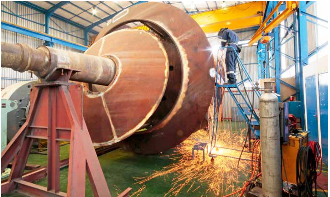
Welder William Gwili is seen in LHM's Fan Service division workshop welding a newly-manufactured fan blade section onto the impeller of the large ID fan from Kendal power station.
