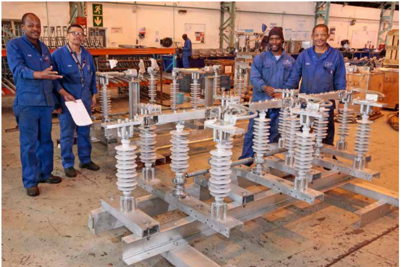
High Voltage Equipment factory staff (from left) Walter Nkadimeng, Foreman; Jimmie Joy, Foreman; Willem Lebenya, Assembler; and Freddie Williamson, Inspector, with the newly-assembled Star Delta portion of the disconnector for the Rustenburg smelter.
