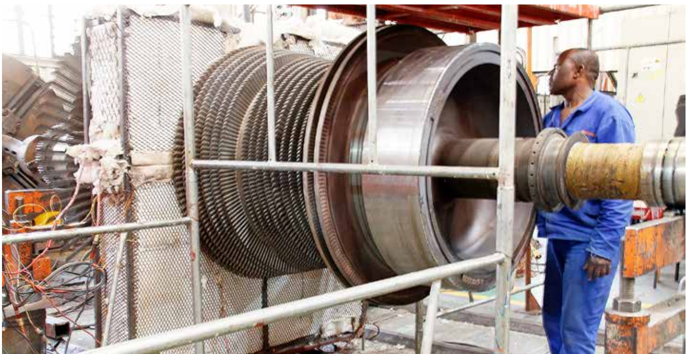
Welding Operator Patrick Luthuli monitors the continuous welding of a large rotor in Metalplus' plant.
