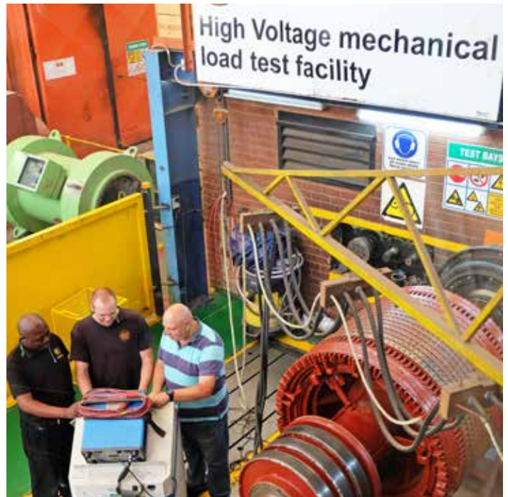
A view from the customer room overlooking M&C's large motors load test facility, showing (from left) Test Facility Foreman Sibusiso Ndlovu, Test Technician Alwyn de Bruin and Test Department Manager Johannes de Lange performing tests on a large wound rotor induction motor rotor.
