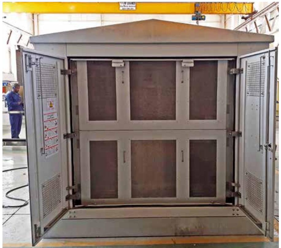
One of MV Switchgear's new PTK's for wind turbines is given a final check over by a technician in the business unit's Knights plant before being dispatched for delivery to one of the new wind farms currently under construction.
