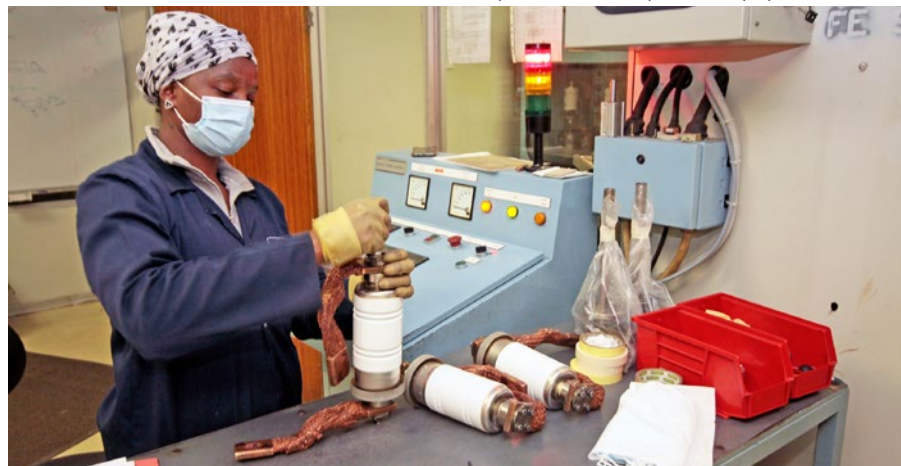
ACTOM VISA (Vacuum Interrupters South Africa) remains the only manufacturer of vacuum interrupters in the southern hemisphere and has recently upgraded its production facilities to manufacture significant volumes of highly customised vacuum interrupters.
