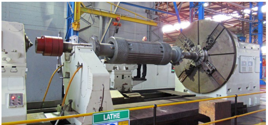
Sappi's 30MW generator rotor undergoing dimensional checks in M&C's 140t precision lathe that takes a 40t work piece, 11m long and a swing of 3.2m.
