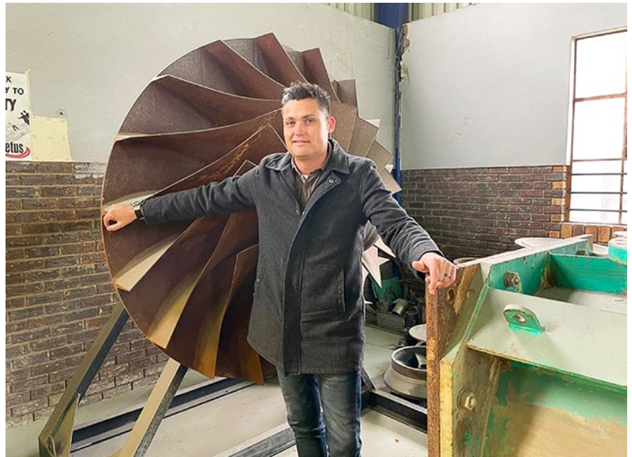
Jurie Erasmus with the rotor and impeller of an Allis-Chalmers single stage overhang compressor from a KwaZulu-Natal pulp mill after completion of repairs on them at ACTOM Turbo's Sasolburg workshop.
