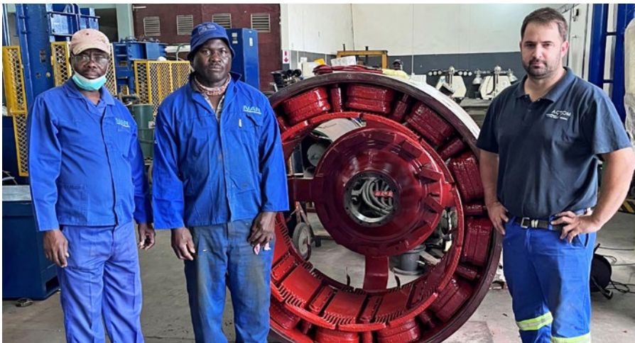
NAR workshop employees (from left) Hoseas Ganaseb, Coilmaker; Titus Igonda, Electrical Fitter; and Aubrey Meyer, Workshop Foreman, after completing refurbishment of the stator of the main generator of a locomotive at the business unit's Walvis Bay premises.
