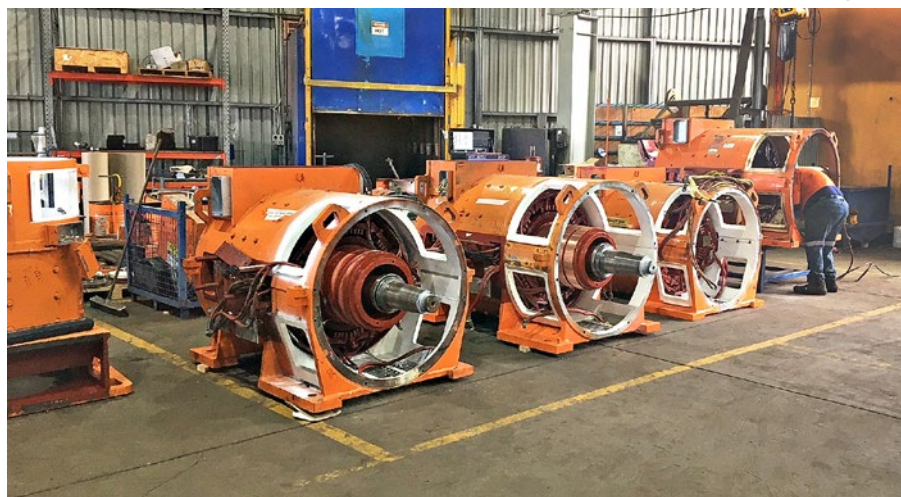
Some of the dragline motors recently brought in for overhaul and repairs at AC Hargreaves' Brisbane workshop.
