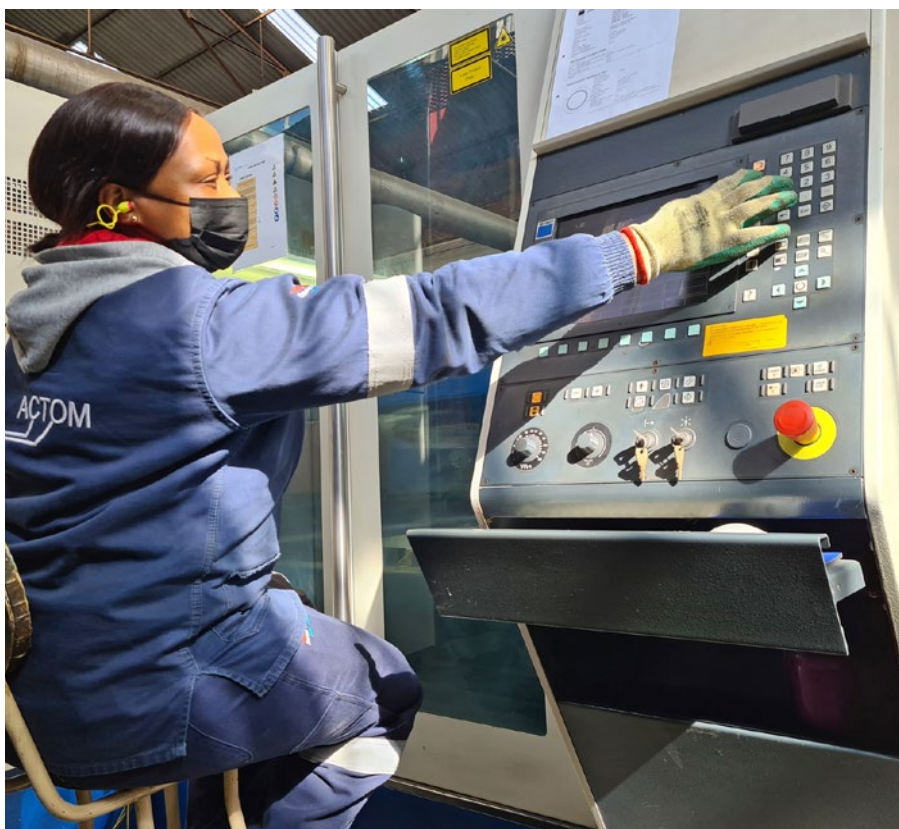
Operator Amelia Mokone is shown profiling laminations for LHM's Rotating Machines division on John Thompson's steel fabrication facility's laser cutting machine in Isando in accordance with the recently arranged cooperative partnership.
