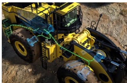
Switched Reluctance equipment layout in a hybrid loader.
