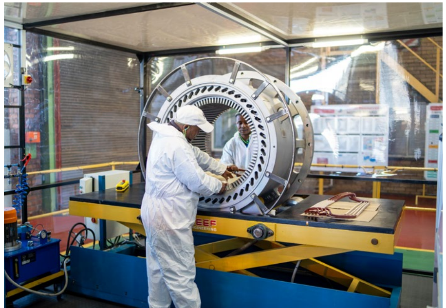
A pair of technicians wind a stator in one of R&M's newly-established clean rooms.
