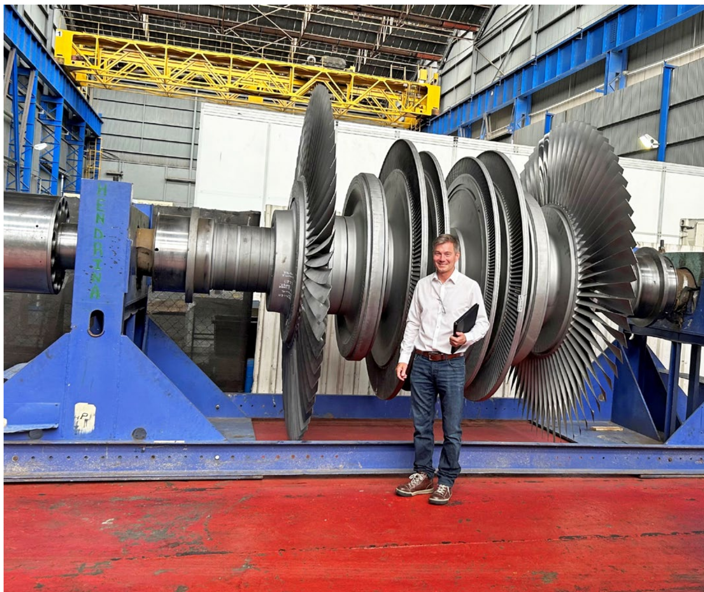
Roman Mornau stands in front of the massive power station turbine rotor after completion of the fine grinding of the unit's blades at M&C's Benoni workshop.
